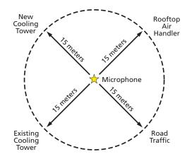
If sound were specified at 15 meters or some greater distance from the sound sensitive location, there is increased uncertainty in the measured data due to other possible sound sources within the 15 meters radius of the sound microphone.
