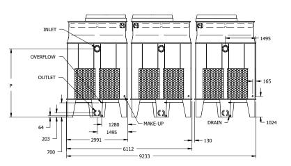
All Inlet and Outlet Connections are: DIN 2576 Flange (Europe) Inlet DN100; Outlet DN100. Make-up MPT DN25; Overflow: FPT DN50; Drain FPT DN50
