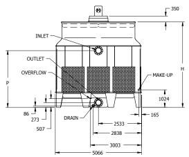
All Inlet and Outlet Connections are: DIN 2576 Flange (Europe) Inlet DN100; Outlet DN100. Make-up MPT DN25; Overflow: FPT DN50; Drain FPT DN50
