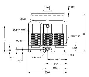
All Inlet and Outlet Connections are: DIN 2576 Flange (Europe) Inlet DN100; Outlet DN100. Make-up MPT DN25; Overflow: FPT DN50; Drain FPT DN50
