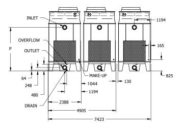
All Inlet and Outlet Connections are: DIN 2576 Flange (Europe) Inlet DN100; Outlet DN100. Make-up MPT DN25; Overflow: FPT DN50; Drain FPT DN50
