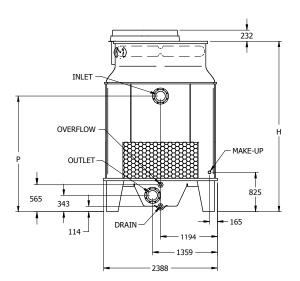
All Inlet and Outlet Connections are: DIN 2576 Flange (Europe) Inlet DN100; Outlet DN100. Make-up MPT DN25; Overflow: FPT DN50; Drain FPT DN50
