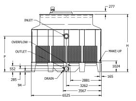
All Inlet and Outlet Connections are: DIN 2576 Flange (Europe) Inlet DN100; Outlet DN100. Make-up MPT DN25; Overflow: FPT DN50; Drain FPT DN50
