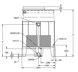
All Inlet and Outlet Connections are: DIN 2576 Flange (Europe) Inlet DN100; Outlet DN100. Make-up MPT DN25; Overflow: FPT DN50; Drain FPT DN50
