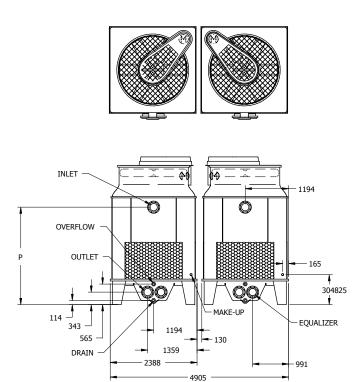
All Inlet and Outlet Connections are: DIN 2576 Flange (Europe) Inlet DN100; Outlet DN100. Make-up MPT DN25; Overflow: FPT DN50; Drain FPT DN50
