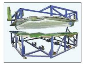
Reinforcement glass fabric loaded into mould cavity
