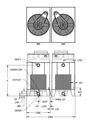
All Inlet and Outlet Connections are: DIN 2576 Flange (Europe) Inlet DN100; Outlet DN100. Make-up MPT DN25; Overflow: FPT DN50; Drain FPT DN50
