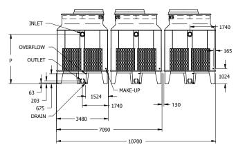
All Inlet and Outlet Connections are: DIN 2576 Flange (Europe) Inlet DN100; Outlet DN100. Make-up MPT DN25; Overflow: FPT DN50; Drain FPT DN50
