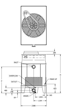
All Inlet and Outlet Connections are: DIN 2576 Flange (Europe) Inlet DN100; Outlet DN100. Make-up MPT DN25; Overflow: FPT DN50; Drain FPT DN50
