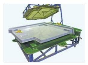
Completed part; removed from mould
