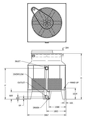
All Inlet and Outlet Connections are: DIN 2576 Flange (Europe) Inlet DN100; Outlet DN100. Make-up MPT DN25; Overflow: FPT DN50; Drain FPT DN50
