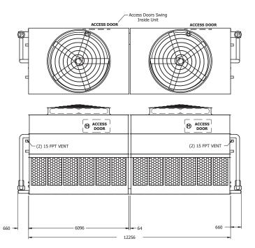
Note: The number of coil connections doubles when the flow rate exceeds 112 l/s on eco-ATWB 12x40 models. This required option is referred to as the High Flow coil configuration.
