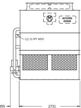
**Note:** The number of coil connections doubles when the flow rate exceeds 56 l/s on eco-ATWB 2.4mx9 models. This required option is referred to as the High Flow coil configuration.
