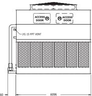
Note: The number of coil connections doubles when the flow rate exceeds 112 l/s on eco-ATWB 24x20 models. This required option is referred to as the High Flow coil configuration.
