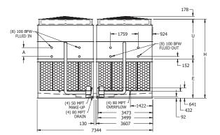
Note: The number of coil connections doubles when the flow rate exceeds 224 l/s on eco-ATWB 24x40 models. This required option is referred to as the High Flow coil configuration. Optional Dual Fan units will have a "-DF" at the end of the model number. Fan kW and weights may vary.
