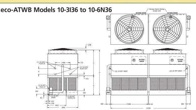
Note: The number of coil connections doubles when the flow rate exceeds 112 l/s on eco-ATWB 10x36 models. This required option is referred to as the High Flow coil configuration. Optional Dual Fan units will have a "-DF" at the end of the model number. Fan kW and weights may vary.
