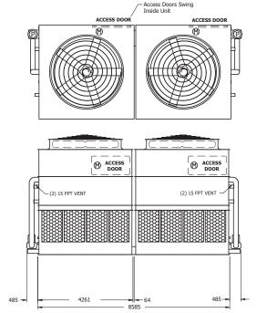
Note: The number of coil connections doubles when the flow rate exceeds 112 l/s on eco-ATWB 12x28 models. This required option is referred to as the High Flow coil configuration.
