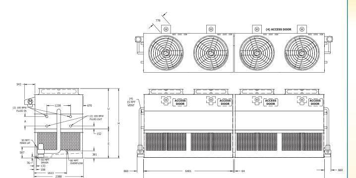
**Note:** The number of coil connections doubles when the flow rate exceeds 112 l/s on eco-ATWB 2.4 m x42 models. This required option is referred to as the High Flow coil configuration.
