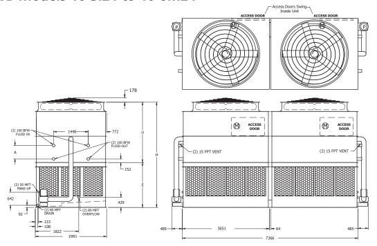
Note: The number of coil connections doubles when the flow rate exceeds 112 l/s on eco-ATWB 10x24 models. This required option is referred to as the High Flow coil configuration.
