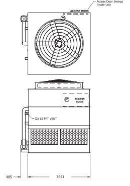
Note: The number of coil connections doubles when the flow rate exceeds 56 l/s on eco-ATWB 12x12 models. This required option is referred to as the High Flow coil configuration.
