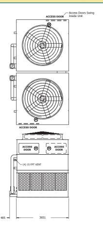
Note: The number of coil connections doubles when the flow rate exceeds 112 l/s on eco-ATWB 24x12 models. This required option is referred to as the High Flow coil configuration.
