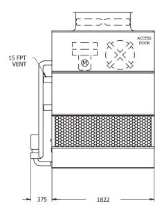
Note: The number of coil connections doubles when the flow rate exceeds 28 l/s on 4x6 models. This required option is referred to as the High Flow coil configuration.
