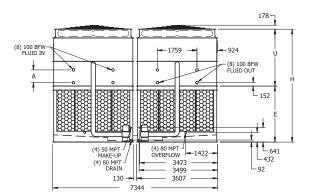
Note: The number of coil connections doubles when the flow rate exceeds 224 l/s on eco-ATWB 24x28 models. This required option is referred to as the High Flow coil configuration.
