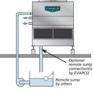
pump, suction strainers and all associated piping, but with an oversize bottom outlet.
