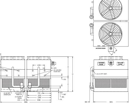
**Note:** The number of coil connections doubles when the flow rate exceeds 112 l/s on eco-ATWB 4.8 m x12 models. This required option is referred to as the High Flow coil configuration.
