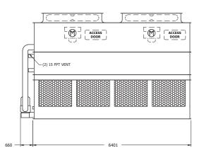
Note: The number of coil connections doubles when the flow rate exceeds 56 l/s on eco-ATWB 2.4mx21 models. This required option is referred to as the High Flow coil configuration.
