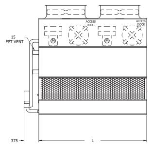
**Note:** The number of coil connections doubles when the flow rate exceeds 28 l/s on eco-ATWB 4x9 and 4x12 models. This required option is referred to as the High Flow coil configuration.
