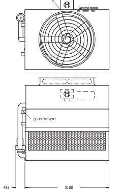
**Note:** The number of coil connections doubles when the flow rate exceeds 56 l/s on eco-ATWB 2.4mx10.5 models. This required option is referred to as the High Flow coil configuration.
