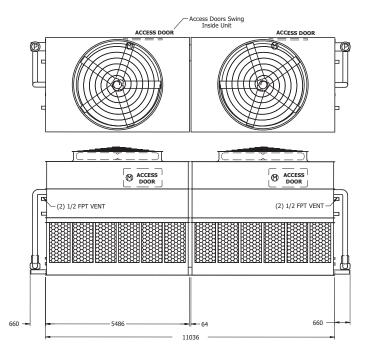
**Note:** The number of coil connections doubles when the flow rate exceeds 112 l/s on eco-ATWB 12x36 models. This required option is referred to as the High Flow coil configuration. Optional Dual Fan units will have a "-DF" at the end of the model number. Fan kW and weights may vary.
