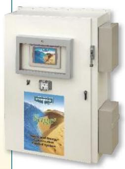
The EVAPCO eco-ATWB closed circuit coolers utilize the optional  $Sage^{2\tau M}$  water and energy conservation control system which controls Dry & Evaporative modes of operation. The control system operates by measuring and analyzing water inlet and outlet temperature simultaneous with ambient dry bulb monitoring in order to minimize the evaporative cooling mode of operation and to save system water. The Sage can also be programmed to operate with a water savings or energy savings priority.
