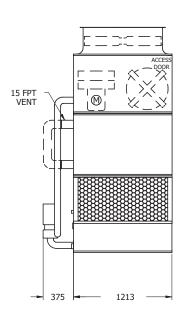
**Note:** The number of coil connections doubles when the flow rate exceeds 28 l/s on 4x4 models. This required option is referred to as the High Flow coil configuration.
