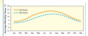
With the increased dry cooling efficiency of the eco-ATWB and the use of the  $Sage2^{\circ}$  Water and Energy Conservation Control System, the eco-ATWB is able to operate dry for more than 30% of the year:
