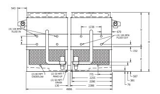
Note: The number of coil connections doubles when the flow rate exceeds 112 l/s on eco-ATWB 4.8 m x10.5 models. This required option is referred to as the High Flow coil configuration.
